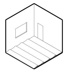
**3.** The loose laying is very important to check the colour uniformity and the absence of defects of the flooring. All claims will be accepted only if the flooring is not yet permanently bonded.
