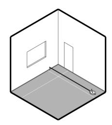
Measure the room and mark the centrelines, planning the laying in a way to reduce cuts and scraps.
