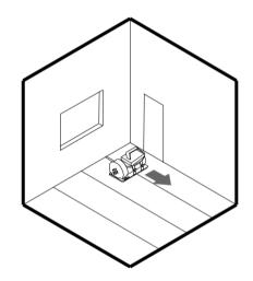
With a grooving tool (manual or powered), create a groove along the joints of tiles or rolls. The groove shall be cut to a depth of 2/3 of the flooring thickness (to a maximum of 2 mm) and a width of about 3.5 mm. Sweep accurately to remove any dust or trimmings from the groove. When laying Granito Elastic the groove shall not affect the underlayer.
