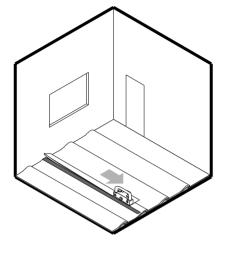
**4.** Perform the seam cutting along the sides and the heads of the rolls (the use of scribers and straight and hook bladed knives is advised to get better results).
