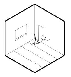
2. Place the sealing rod into the speedweld aperture, press the rod down into the groove and proceed at the right speed keeping the speedweld toe parallel to the rubber surface.
