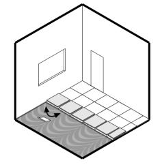
Tip over a row of tiles at a time. Spread the adhesive with the proper notched trowel as advised by the manufacturer.
