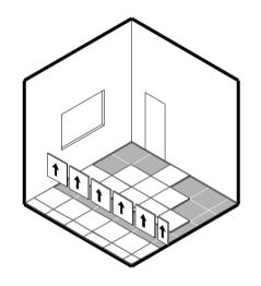
Loose lay the tiles (without adhesive) starting along the centrelines and following the arrows printed on the back of the tiles taking special care to the alignment of joints and/or pattern.
