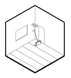
After the laying, the use of a floor roller is recommended to ensure a perfect contact with the substrate.
