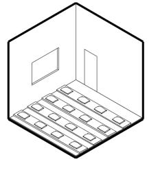
In case adhesive with long tackifying time are used, apply weights along the joints (bricks, sand bags, etc.).
