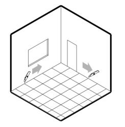
3. Check the uniformity of colour and the absence of defects. The perimeter tiles will require to be trimmed off to be ready for bonding.
